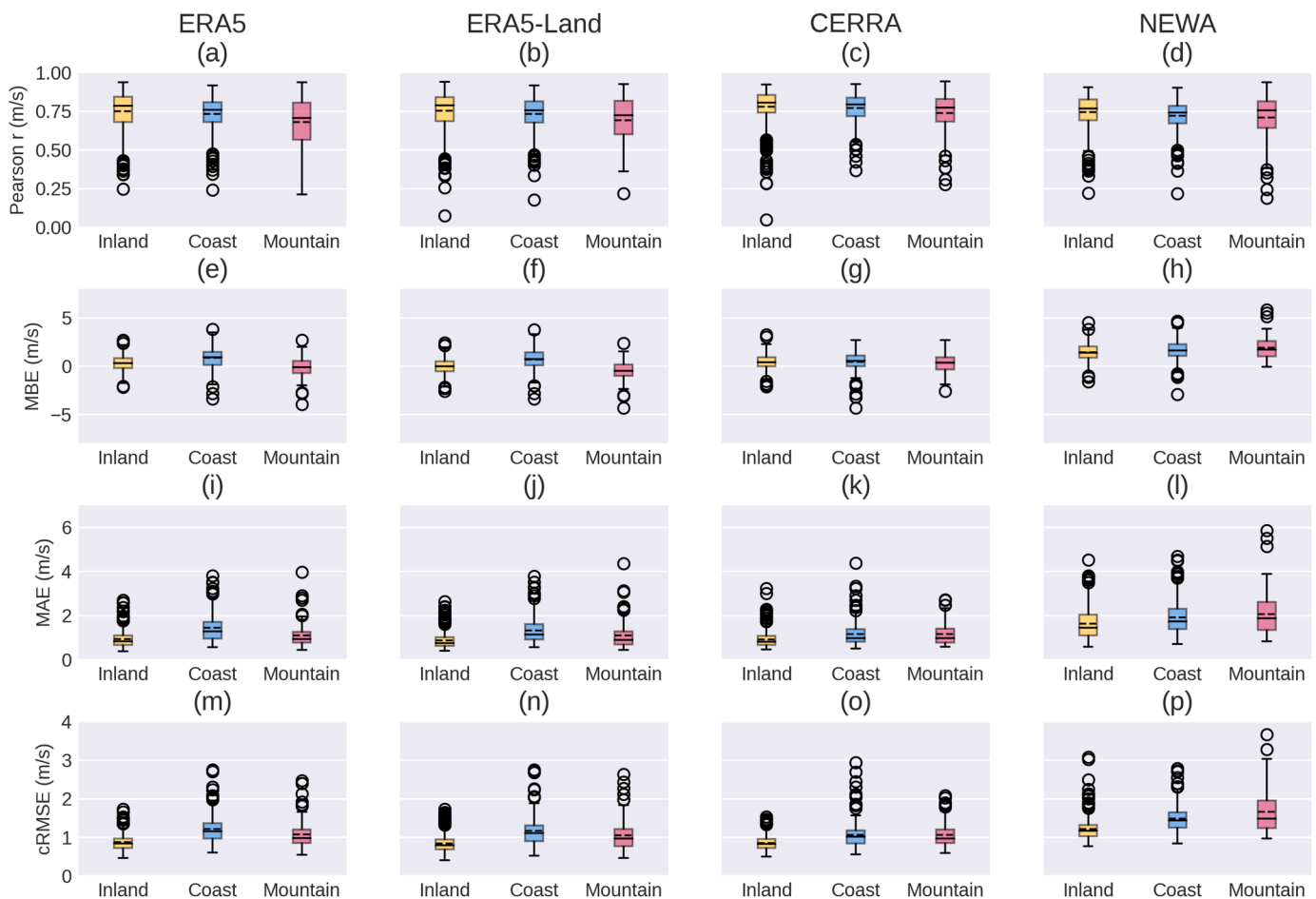
Fig. 5. Significant Pearson correlation ( p < 0.05 ), MBE, MAE and cRMSE between weather stations and ERA5, ERA5-Land, CERRA and NEWA according to their classification into coast ( N = 220 ), inland ( N = 403 ) and mountain ( N = 125 ) for 1/Jan/1990–31/Dec/2018 (Each box shows the interquartile range (25th–75th percentiles), with horizontal lines representing the median (solid) and the mean (dashed). Whiskers indicate extreme NSWS (1.5xIQR), and circular markers highlight stations beyond this range).
